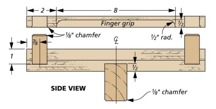
I also routed a finger grip along the underside edge of each tool platform. Then it's just a matter of attaching the bench-mounted tools to the platforms.
