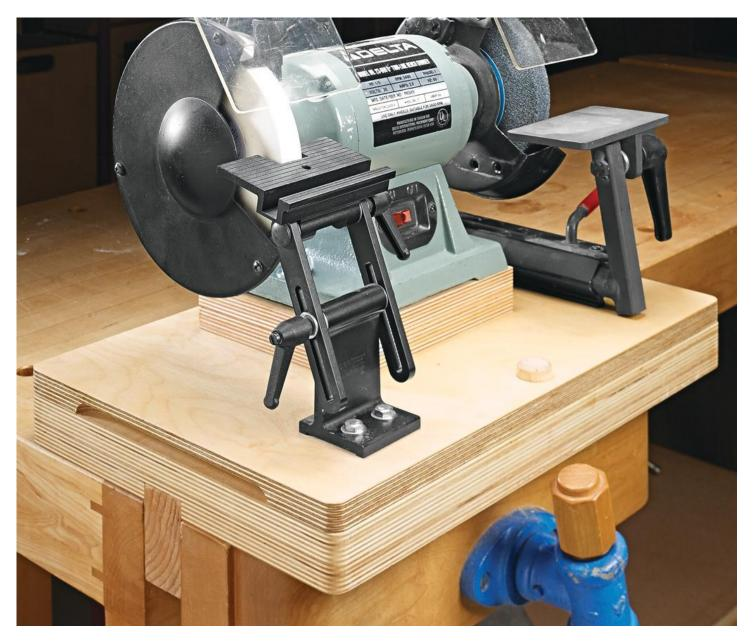
Workbench space is at a premium in my shop. To make the most of the space I do have, I wanted an easy way to use smaller bench-mounted tools (my grinder and machinist's vise) in the same location. What I came up with is this interchangeable work platform that clamps into the face vise on my bench.
